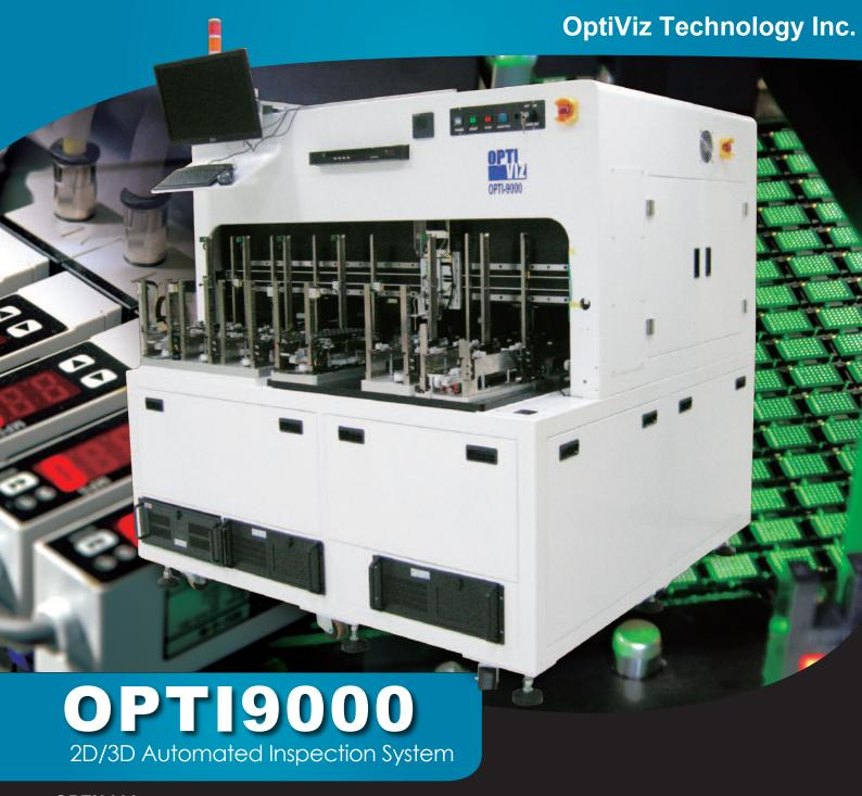
**OPTI9000** offers high speed, in-tray, 2D and 3D inspection. Providing both high throughput and high resolution, OptiViz's proprietary 3D laser scanning technology and 2D inspection modules are the ideal combination for speed and accuracy while balancing cost of ownership.
